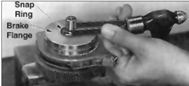
Figure 5-6. Remove Snap Ring From Load Brake Shaft
