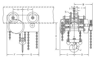
\* Applies to geared units only \*\* At closest point of contact This unit is beam specific (non-adjustable) Dimensions shown are accruate for "S" & "W" beam shapes
