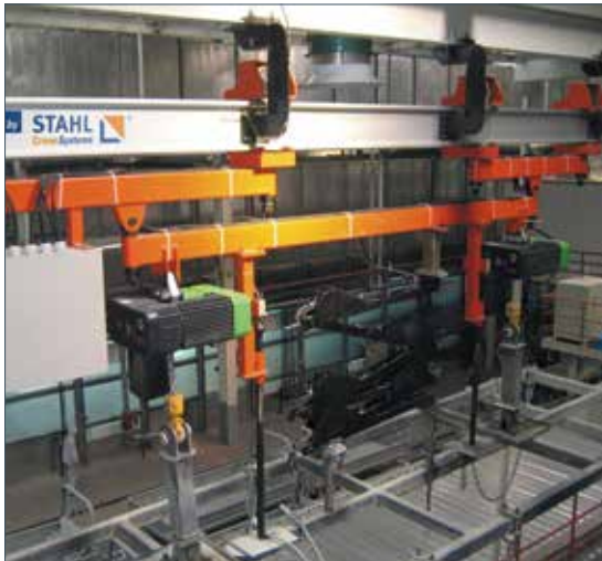
In a coating plant for the automotive industry in China, 48 specially designed ST chain hoists operate at very high humidity levels.
