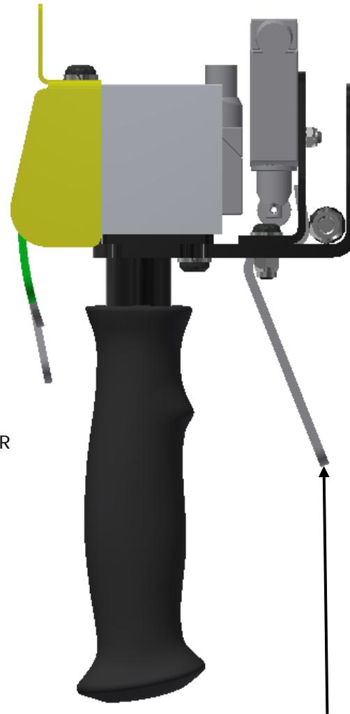
4-PIN MICRO-SINGLE POLE LIMIT SWITCH WITH 1 NORMALLY OPEN AND 1 NORMALLY CLOSED CONTACTS FOR USE WITH ANY 24 VDC DEVICE
