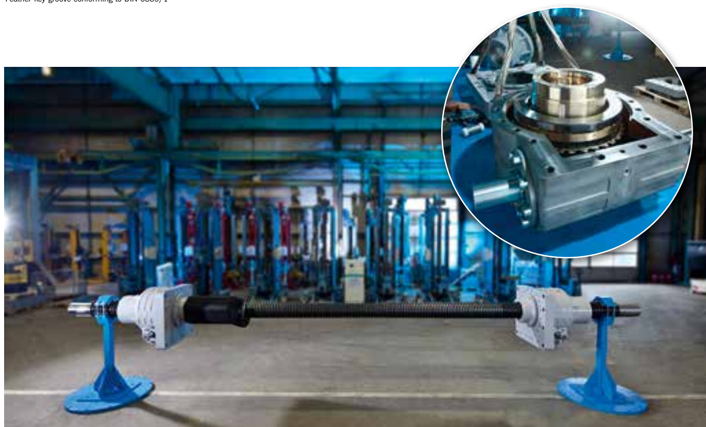
Assembly area Pfaff-silberblau: Special design screw jack SHE 200.1 with 8 m long screw and protection boot. Design for a static load of 400 tons.
