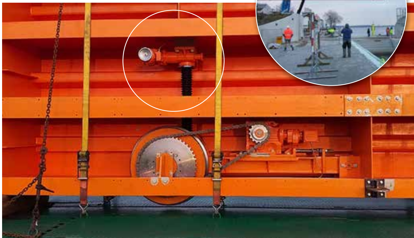
Fig. 1: Close-up view of the gate with the SHE 25 from Pfaff-silberblau for adjusting the travel wheel (copyright: ARGE HPI/hpl Greifswald) Circular image: Detailed view of the gate with the SHE 25 from Pfaff-silberblau for adjusting the impeller (Image rights: ARGE HPI/hpl Greifswald)
