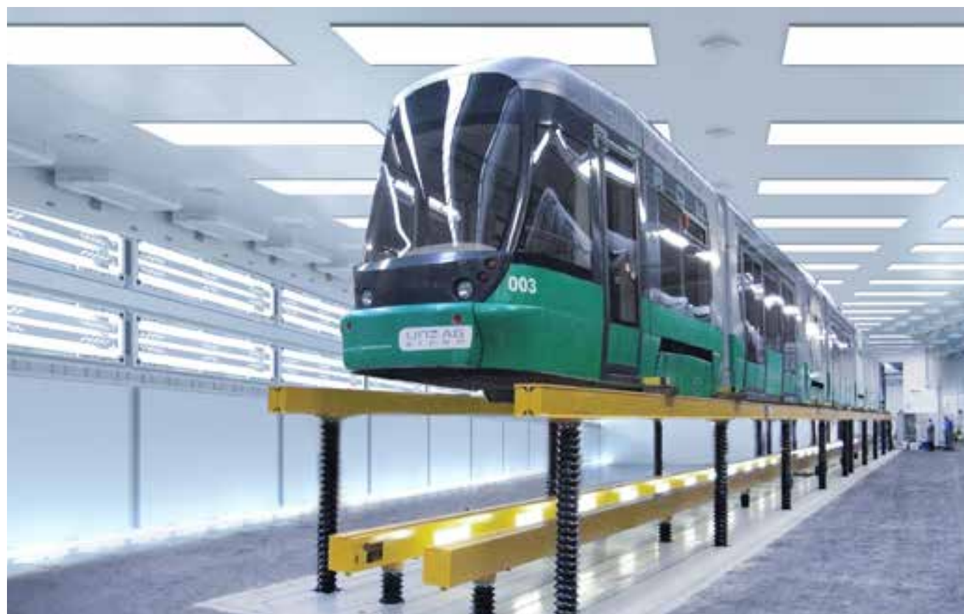
Pfaff underfloor lifting system with SHE 25 worm gear screw jacks designed according to DIN EN 1493
